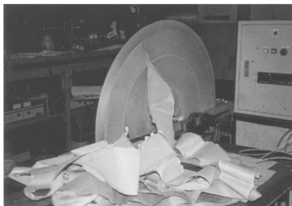
Fig. 3. Photograph of the aluminium disc cathode and zinc deposit coil.
